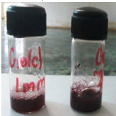
Fig 1: Appearance of purple color in solutions of 1mM and 2mMHAuCl 4 indicating the synthesis of gold nanoparticles
