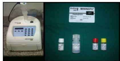
Figure 3: Mininephplusnephelometer and haptoglobinkit (swipecard, antiserum, buffer, controls)
