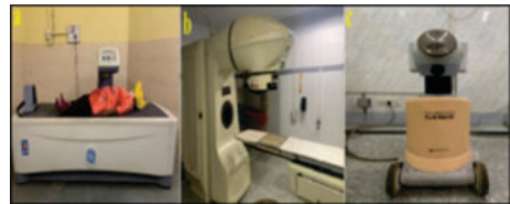
Figure 1: a) DEXA scan machine (Lunar Prodigy Advance Machine); b) Teletherapy cobalt unit (Theratron 780E); c) Brachytherapy Unit
