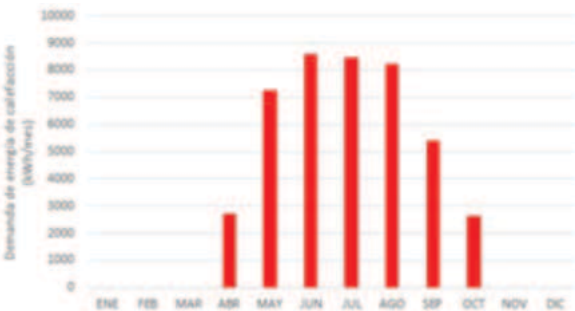
Source: own. Fig. 12: Heating energy demand in kWh/month calculated for T Bcal = 20°C, original situation.
