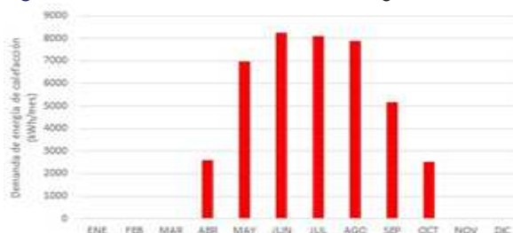
Source: own. Fig. 7: Heating energy demand in kWh/month calculated for TBcal = 20°C, original situation.
