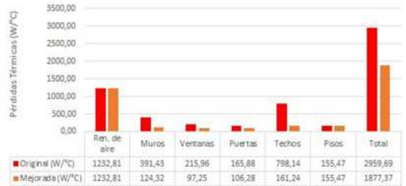
Source: own. Fig. 13: "Eluney" nursery school. Comparison of original and improved version. Winter.
