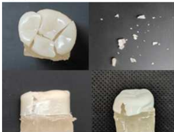
Figure no. 3: Fractured Zirconia crown, Figaro crown and Bioflx crown
