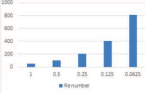
This shows that a wide range of pipe diameters could be used to give Reynolds numbers below 2000, i.e. streamline flow.
