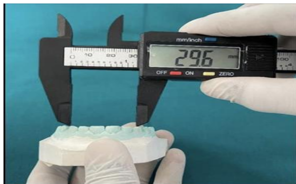
Figure 1. Measurement of Intercanine Width Using a Digital Vernier Caliper
