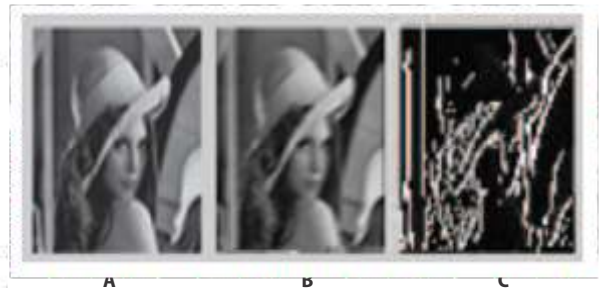
Fig(7). (A) Input image, (B) Low pass filtered image, (C) High pass filtered image
