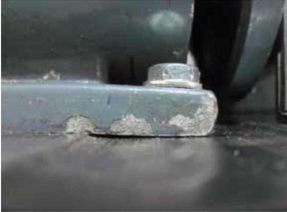
**Figure 10. MOTOR BASE WITH SOFT FOOT**
