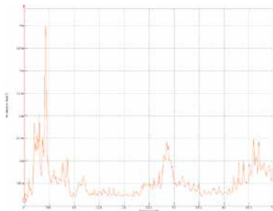
Figure 5.1 Sample Vibration Spectrum (Refer Table 6.1 Case 5 Expt. No. 1)
