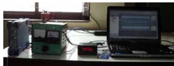
Figure3.3. FFT Analyzer (OROS 34)
