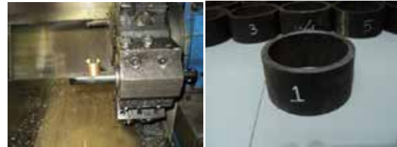
Figure 4.2: Boring bar installation Figure 4.3: Sample workpiece
