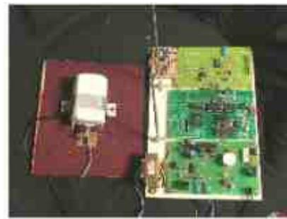
Fig. 5 Motor & Power Control Unit
