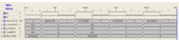
Fig.14. Output waveform of Serial to Parallel converter
