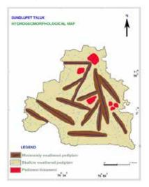
In addition at limited spots around Gundlupet taluk we carried out Schlumberger Resistivity Sounding Survey and the aquifer depths have been found around 150 mt to 200 mt of depth. Finally all these thematic maps have been analysed and a composite hydrogeomorphological map has been generated as shown in appropriate places.
