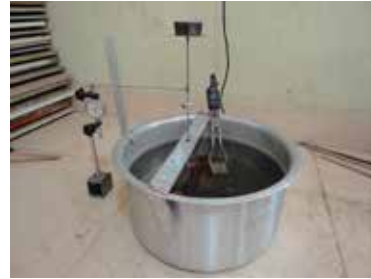
Figure 5: Experimental set up for Heat Deflection Test
