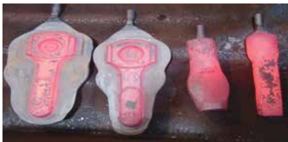
Fig.2: Schematic showing the principle of forging a connecting rod
