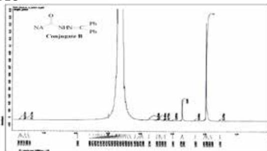
**Figure 4: 1H NMR spectra of conjugates B recorded in D2O**
