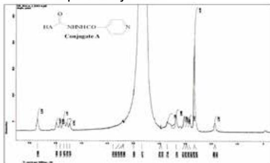
**Figure 3: 1H NMR spectra of conjugates A recorded in D2O**
