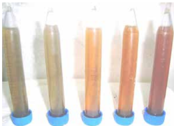
Figure3. Picture showing the samples after rapid biosynthesis of silver nanoparticles using Parthenium hysterophorus
