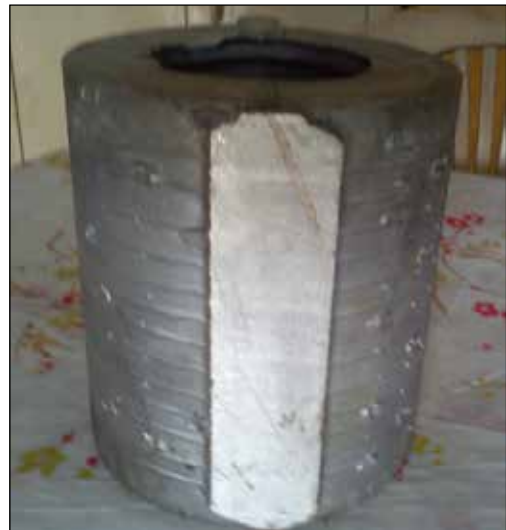
Figure 1.2 Defected shell core drum
