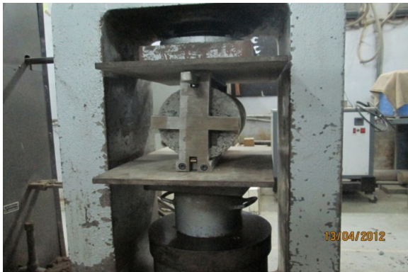
Fig-1 Splitting Tensile Strength Set Up
