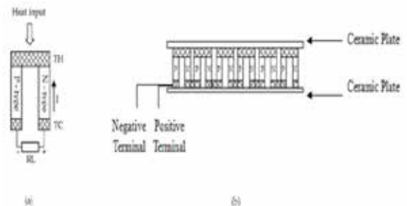
Figure 1: (a) Schematic diagram of a single thermoelectric couple, (b) Side view of a thermoelectric module.
