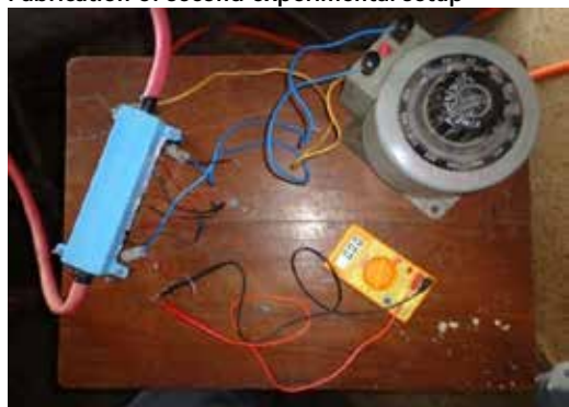
Figure 4: Experiment on Separate setup with heater and Dimmerstate.
