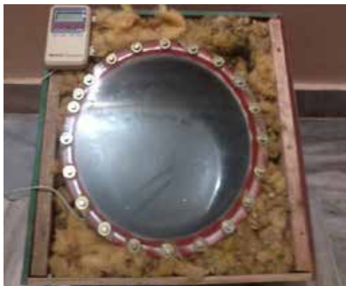
Fig.1. Source part inserted in double insulation of Glass wool and Wooden Block
