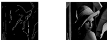
Fig.3. Image processing (a) After Averaging Template, (b) After Averaging and Edge Detection
