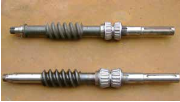
Fig: 4 Old (top) and Modified (bottom) Shafts
