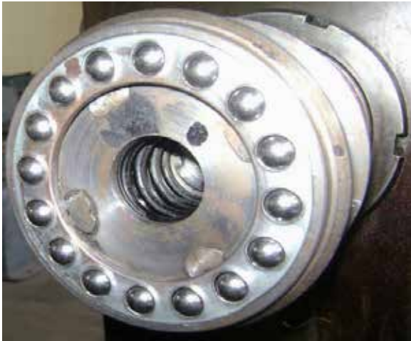
Fig.3: ball burnishing tool engaged with Milling machine
