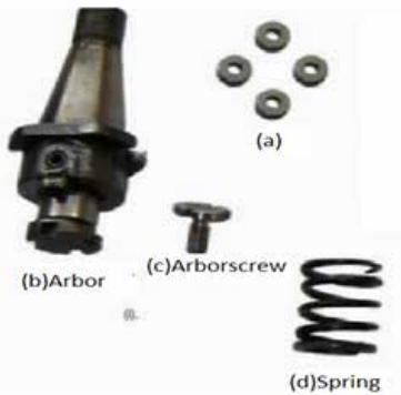
Fig. 4: Burnishing Tool Parts and Work piece
