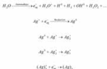
Scheme 1: mechanism of silver ion reduction by γ radiation.
