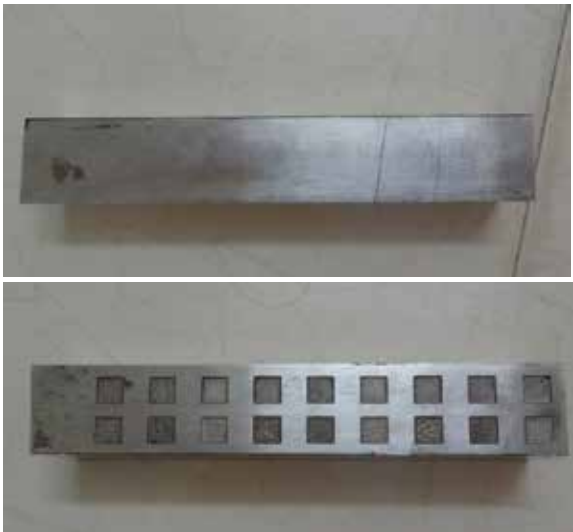
Figure 4. EN31 material before machining and after machining
