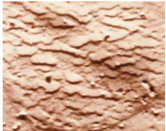
Fig.4(b): Optical micrograph for 0.5\mu\text{m} InSb films
