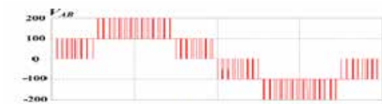
Fig. 5 Simulated waveforms of phase voltage V AB of inverter stage [Scale: 100V/div]
