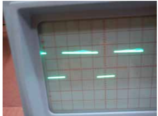
Fig.14 Pulse generated from the driver unit (12V)
