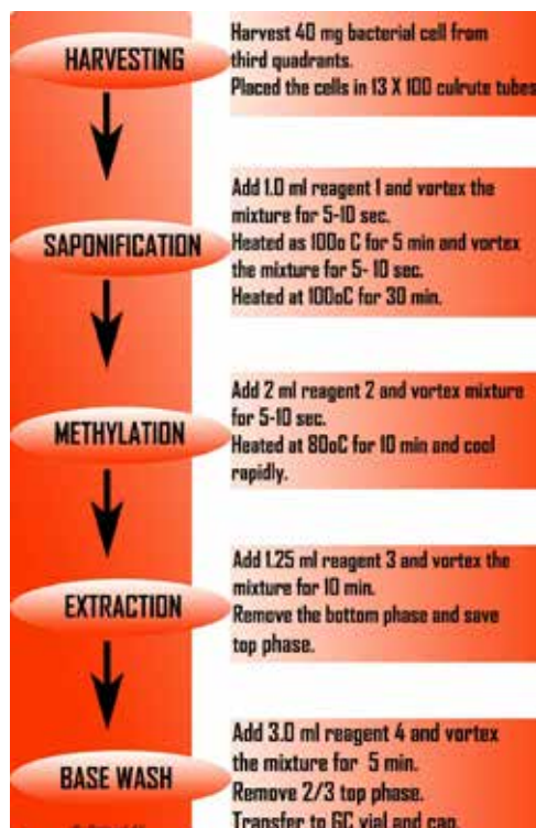
Fig. 1: Flow chart explains the extraction process of fatty acids.
