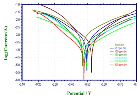
**Figure 3: Tafel polarization plots of MS in 1 M HCl solutions with various concentrations of LP drug.**
