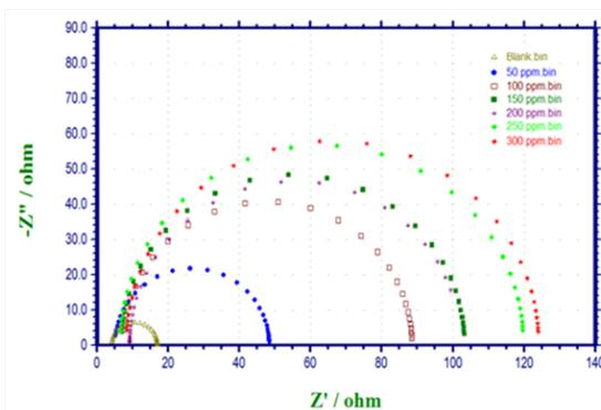
**Figure 2: Nyquist plots of MS in 1 M HCl solutions with various concentrations of LP drug.**
