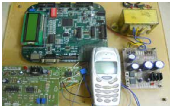
Figure 1: FPGA connected with Nokia phone.
