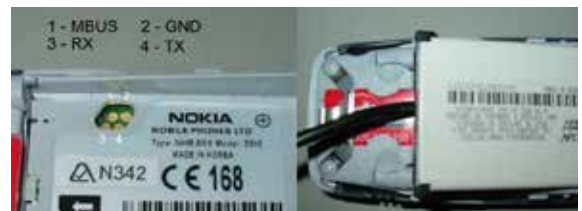
Figure 2: FBUS connection in Nokia phone.
