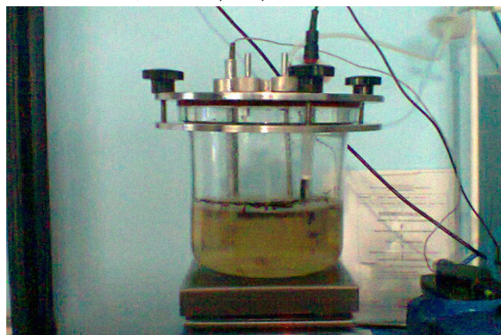
Figure 1: Fermentation of Amylase enzyme using Aspergillus niger (Lab scale fermenter, BioEra 5L, College of Computer Science and Technology, Latur)
