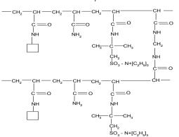
Scheme- 1. Poly (N-cyclohexylacrylamide-co-acrylamide/ AMPS Ionic Liquid) Hydrogels
