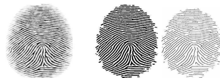
Figure 2: (a) Original Fingerprint (b) Binarized image (c) after thinning
