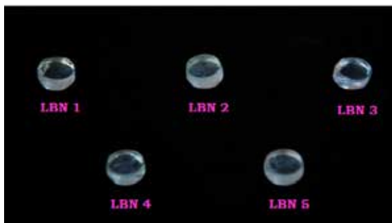
Fig. 2.1 Glass samples of LBN system
