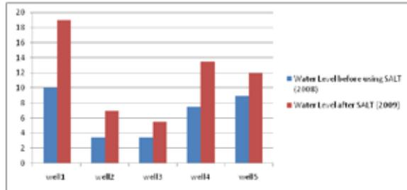
Above graph clearly represent a hike in water level after applying SALT technology over the sloppy area of that hill. To analyze the impact of these efforts on ground water level one tail t-test is conducted. Following hypothesis is taken for the same purpose.
