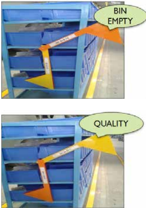
Figure 2- Kanban flag indicating bin empty and line stoppage
