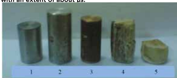
Figure 5: Samples for which the speed of sound was measured. 1)Fe, 2)Al, 3)Cu, 4,5)hard bone.
