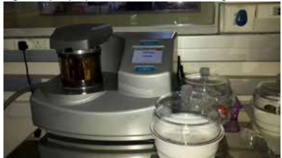
Fig4.Gold coating after sample preparation before SEM testing [2]
