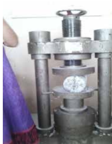
Fig 1: Split tensile strength test
