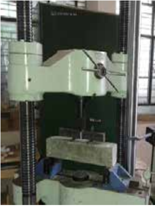
Fig. 2. Flexural Strength test
