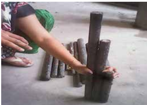
Fig .2.3. Hollow stiffened steel tubes with different length such as 238.2mm, 421mm, 538mm with 26.9mm diameter &1.6 mm thickness.
