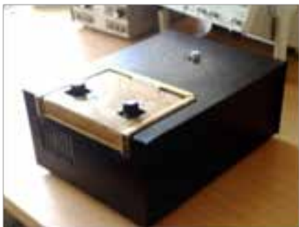
Figure 5: STM mechanical components sitting on the vibration isolation system inside a metallic box.
