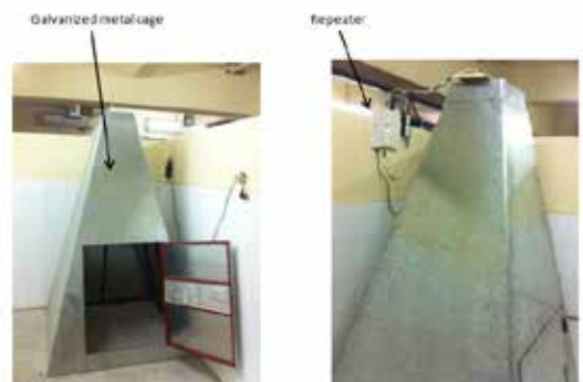
Figure 1: The experimental device for the production of the signal GSM in the 900-1800 MHz band (Casablanca Ben M'Sik Science Faculty)
