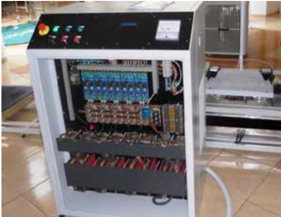
Figure 8. Demonstration of the complete IPT system for static and on-route charging of EV's – Converter "4 in 1"
