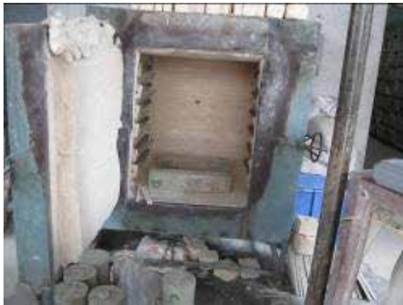
Fig. 1 Furnace for heating the samples
