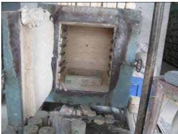
Fig. 1 Furnace for heating the samples
