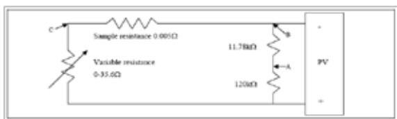
Fig.(3) PV logging system circuit
