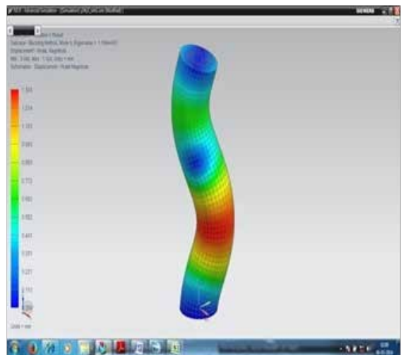
APPLYING LOAD ON TOP FACE OF CONCRETE FILLED STEEL TUBE
